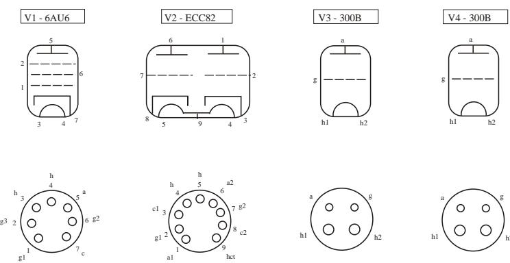
Views from underneath valve or valve holder
